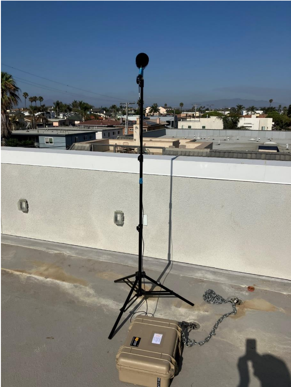
Figure 1: Installation photo of the rooftop continuous monitoring 2250 sound level meter at 951 Seacoast Dr.
