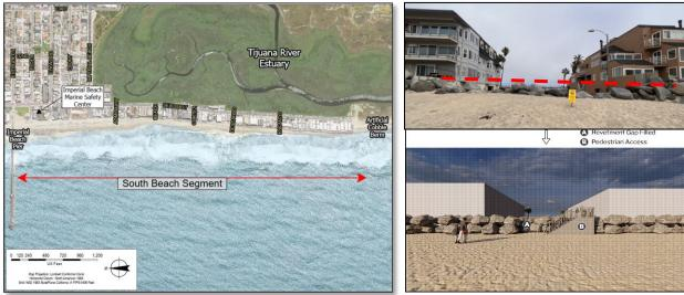
Segment 4: (Green) Floodwall on the estuary side of south Seacoast Drive that is adaptable with an elevated boardwalk and (Yellow) Living levee with elevated path adjacent to the Seaside Point Neighborhood
