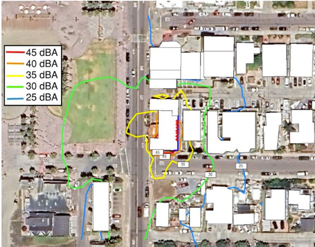
Figure 5: Sound contour lines with mitigation measures in place. Sound receiver heights are set to 1.5 m. Red plus signs indicate proposed speaker locations. Blue line at building edge represents the fully extended/raised parapet.
