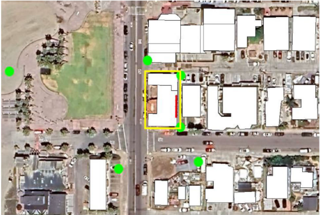
Figure 3: Layout of computer-modeled sound sources and sound receivers for project site and its surroundings. Project site is outlined in yellow; sound sources are denoted by the red line; modeled sound receivers are marked by green circles.
